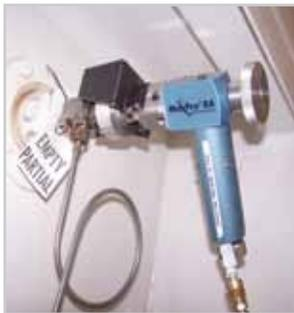
The air supply hose has a safety swing coupling to ensure a secure connection between actuator and gas supply, while helping to prevent kinks or tangles in the hose. The length of the air supply hose assembly is custom made at time of order.
